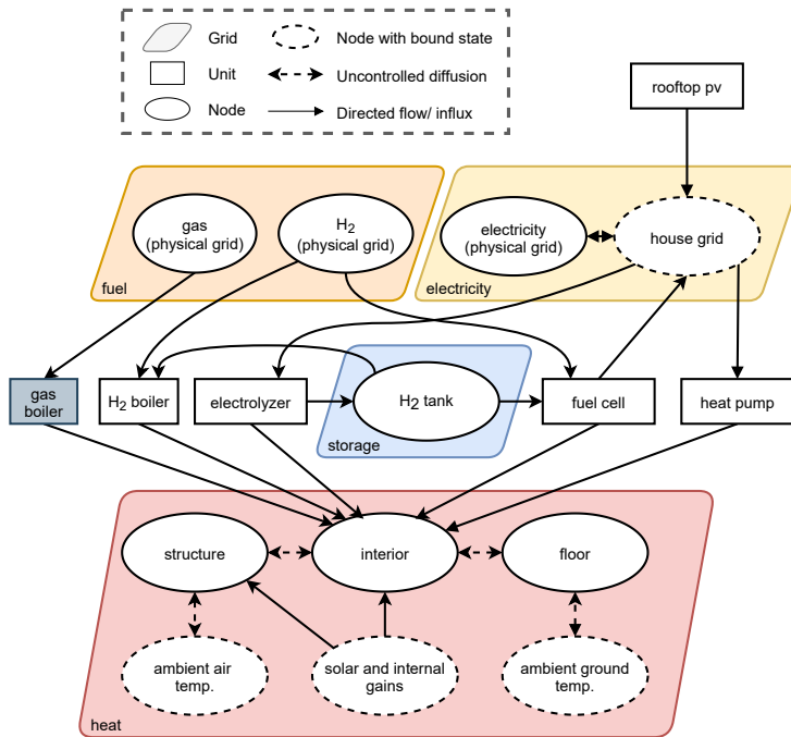
Figure 1: Schematic representation of the building model. Note that the gas boiler is the only unit present in the model from the beginning. All other units can only be utilised upon investment.
