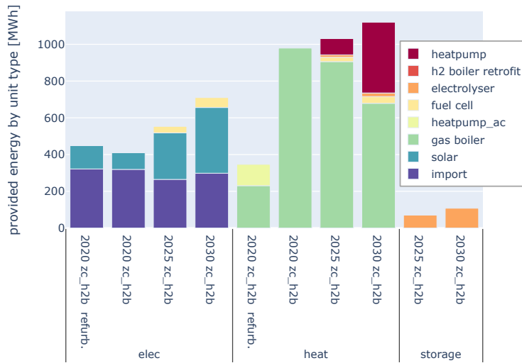
Figure 5: Energy generation for each grid by unit type
